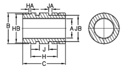
For o-ring  $= 9.7 \times 1.3$ = 5.027999999999996 A max A min = 5.01Η = 12 B max = 12 HA = 1.139999999999999 B min = 11.98199999999999 HB = 11.5 J = 5 Bush weight kg = 0.004C max = 22 JA = 2 C min = 21.74599999999999 JB = 9.86Ret ring part no (DIN 471) = 12 Concentric mm = 0.0254
